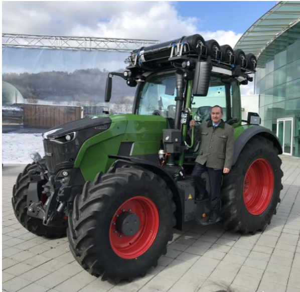
Fendt, Germany - hydrogen fuel cell powered tractor, H2ARGAR research project
