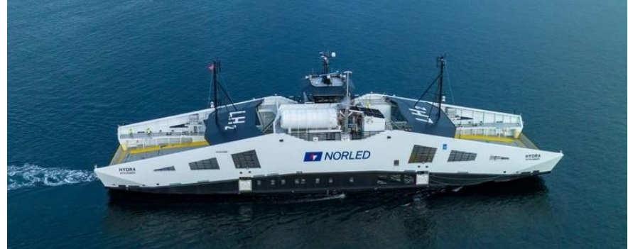
Hydra hydrogen powered ferry, Norway
